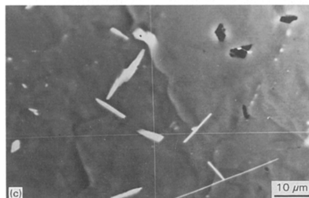
Figure 10 Transformation of the \alpha_c -AlFeSi intermetallic phase at 630 °C. (a) As-cast condition; (b) after 4 min; (c) after 8 min.
